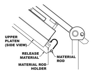
3. Holding the bottom of the release material sheet in place, gently pull the sheet toward the front of the platen.
